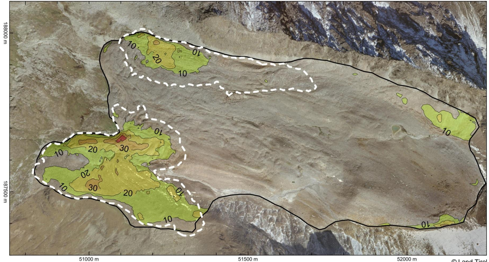
Mean annual horizontal flow velocity for the time period 2003-2010 , isotachs ( \text{cm a}^{-1} ), significance level at 10 \text{ cm a}^{-1} ( 3\sigma ).
